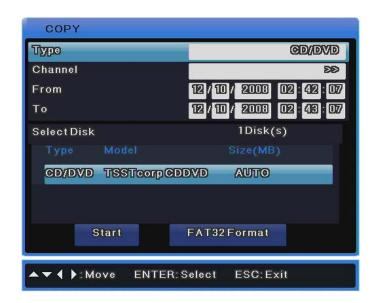
The SVR-945 is not equipped with a DVD device so you must connect the unit with an external backup device. Connect an external backup device to the USB or eSATA port, execute copy and select CD/DVD. On the media list, a CD/DVD device whose type is [Ext] is displayed. Select the device and make a copy in the same way as other models.
